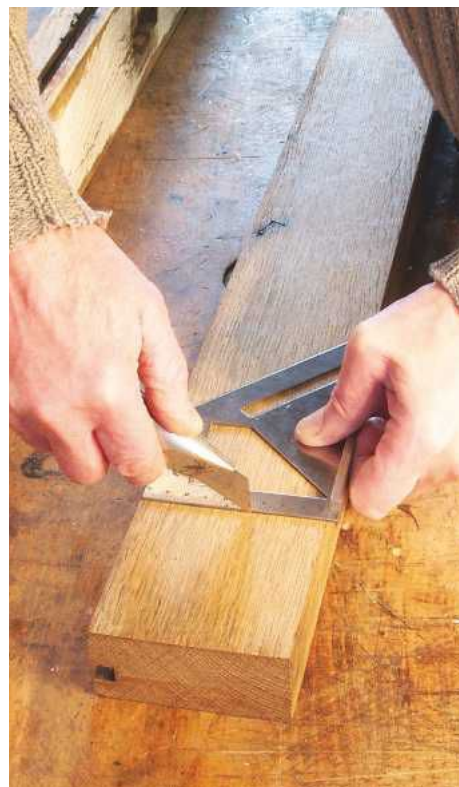
▲ Pic.8 Offer the square up to the blade and run the line across the rail
